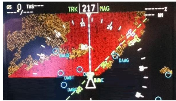
Typical map display with terrain relative height indicated with different colors green-amber-red
