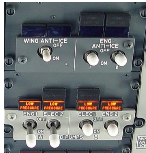
The Hydraulic Pump switches can be mistaken for Engine Anti-Ice switches
