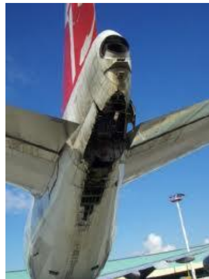
Tailstrike on a 747 beyond economical repair due to a mix up of ZFW and takeoff weight
